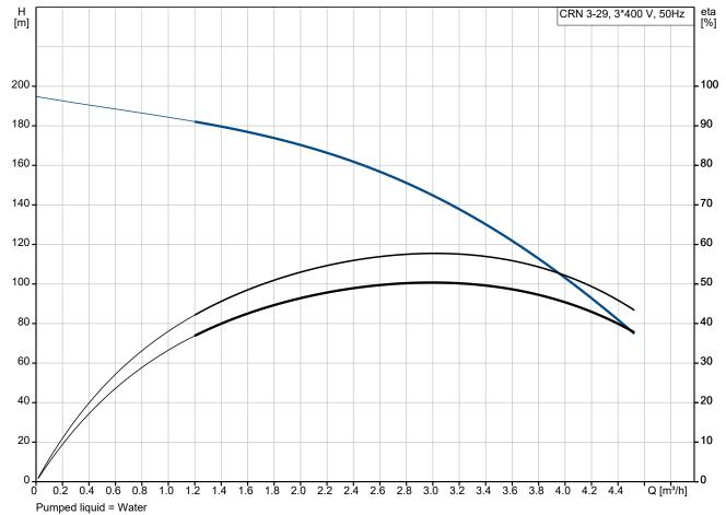
Liquid temperature during operation = 20 °C
