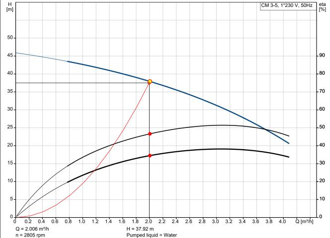
n = 2805 rpm Liquid temperature during operation = 20 °C Pumped liquid = Water Density = 998.2 kg/m<sup>3</sup>
