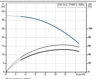
Pumped liquid = Water Liquid temperature during operation = 20 °C Density = 998.2 kg/m³
