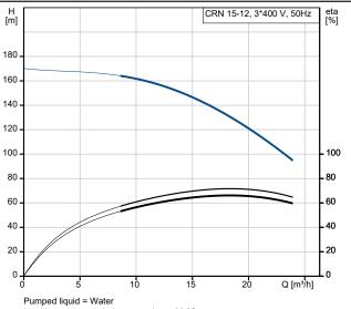
Liquid temperature during operation = 20 °C
