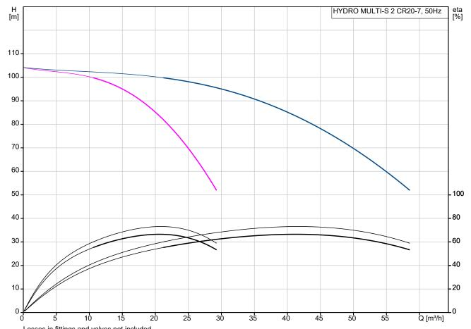
Losses in fittings and valves not included Pumped liquid = Water Liquid temperature during operation = 20 °
