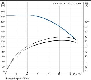
Liquid temperature during operation = 20 °C Density = 998.2 kg/m<sup>3</sup>
