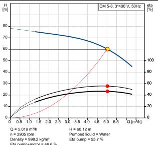
n = 2905 rpm Density = 998.2 kg/m³ Eta pump+motor = 46.6 %
